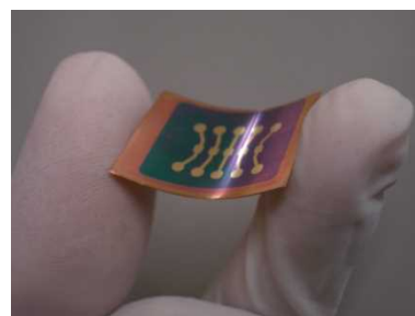
Flexible transistor fabricated in his laboratory.
