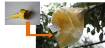
Environmental sensing by a micro sensor installed in a pear sack.
