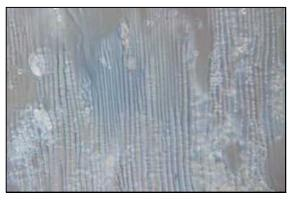
Typical optical pattern observed in shear flow of smectic liquid crystal
