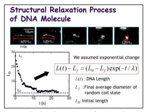
Structural relaxation process of DNA polymer affected with gap size in a micro channel
