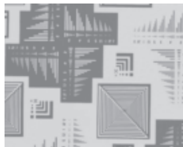
Fig.2 Optical micrograph of pDDMA-DNMA LB films with 11 layers on a silicon plate irradiated with a deep UV light
