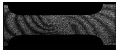
Interferometric fringe pattern during serration of aluminum alloy
