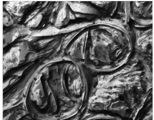
Lamellar crystals of the monodisperse centrally-branched alkane C_{96}H_{193}.CH(C_4H_9) . C_{94}H_{189} form cylindrical tubes at high crystallization temperatures with all branches on the outside of the tube. Surface packing considerations must, therefore, outweigh distortion of the crystal lattice
